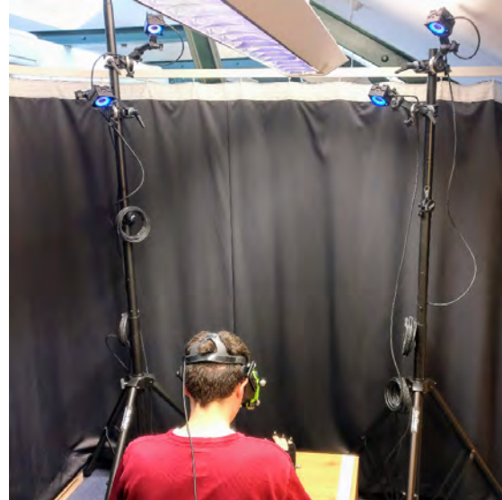
(b) Positioning of the OptiTrack infrared cameras.
